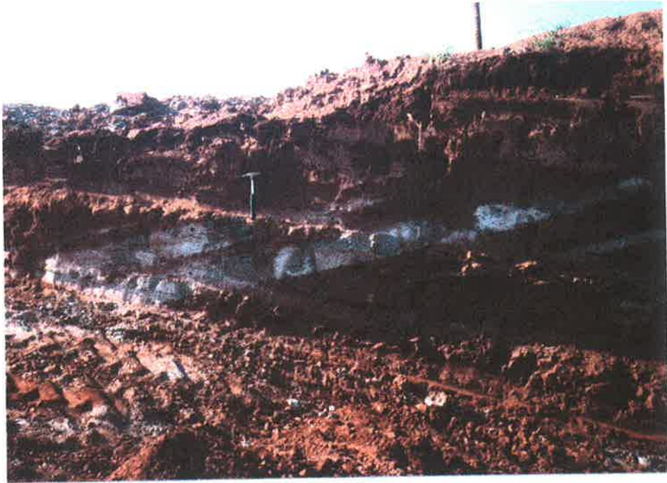
Photograph 5 - View of the conglomerate bed exposed along the active area trench. The conglomerate is composed of loosely cemented gravel and sand.
