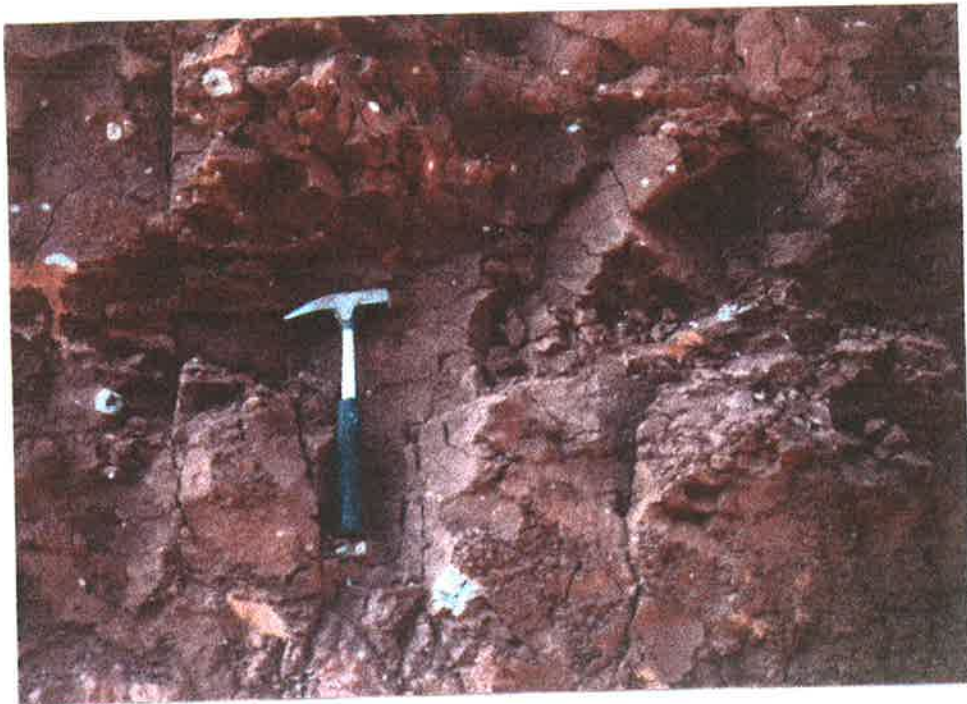
Photograph 6 - Closeup View of exposed trench side wall showing the typical characteristics of fractures in the red beds.
